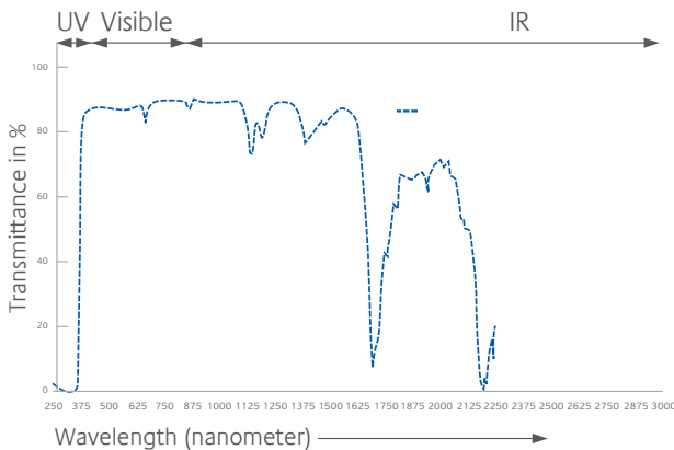
FIGURE 6 LIGHT TRANSMISSION SPECTRUM OF LEXAN SHEET
